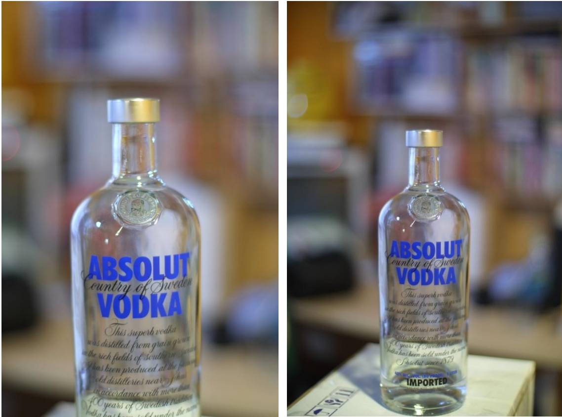
Figure 19: Carl Zeiss 50mm/1.4 in Yashica/Contax mount on a Fujifilm X-E1 camera. The left image is with a simple mechanical adapter, the right image with the Speed Booster. Same distance, but different exposure time because of the increased speed. Left image is 50mm f/1.4 and 1/30s, the right image is 35mm f/1.0 and 1/60s. Obviously, the magnification is different.
